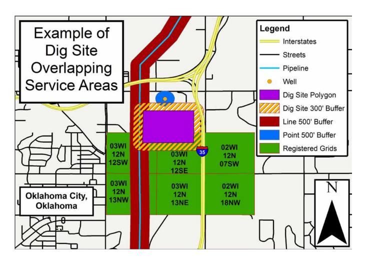
\*Locate requests are generated when the excavation site polygon overlays the asset polygon.
